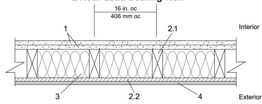
1. Gypsum Board (Interior): Two-layers Type C USG Firecode® C Core complying with ASTM C1396, minimum <sup>5</sup>/<sub>8</sub>-inch-thick (15.9 mm), 4 feet (1.2 m) wide applied vertically, fastened to framing. Face layer joints staggered with base layer and covered with paper tape and joint compound.
