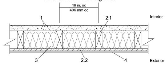
Gypsum Board (Interior): Two-layers Type C USG Firecode® C Core complying with ASTM C1396, minimum <sup>5</sup>/<sub>8</sub>-inch-thick (15.9 mm), 4 feet (1.2 m) wide applied vertically, fastened to framing. Face layer joints staggered with base layer and covered with paper tape and joint compound.
